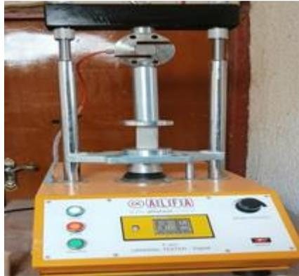
**Figure 4** UCS test device
